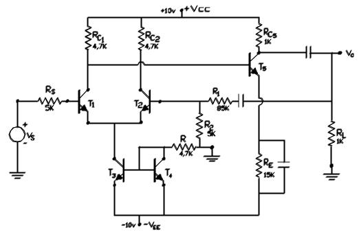
$$I_{CQ1-2} = I_{CQ5} = 1 \text{ mA} - r'_b = r'_c = 200 \text{ Ohm}.$$
